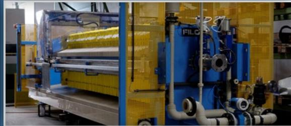
The automatic drip tray can be driven hydraulically or pneumatically. Can be designed as a slewing or shearing device.
