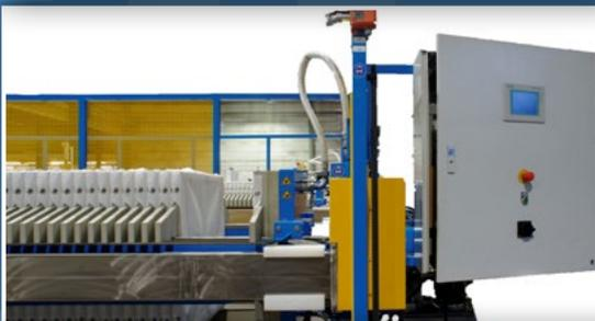
Our automatic filter press is operated through PLC controls. Visualization is done on a key screen or a touch panel.
