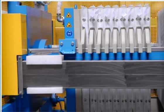
The automatic plate transport is driven hydraulically and regulated by a pressure sensor. The low-maintenance plate transport carriages are guided on lateral stainless-steel profiles.
